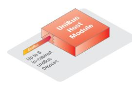
UniBus Devices are designed for installation within the same enclosure as the UniBus host module. A UniBus host can interface a maximum of six UniBus devices in any combination, provided they are all within the intended functionality of the host module
