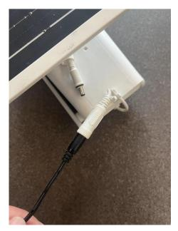
After fully charging, unplug the external power cord and connect it back to the original solar panel wiring.
