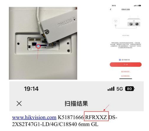
In addition, you can also press and hold the reset button of the device body directly until you hear that the device is activated, use SADP to search for the device IP, assign an IP to the device, and modify the password.
