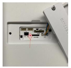
Press and hold the device Reset key until the indicator light flashes blue, and the device will automatically activate and launch EZVIZ cloud. The default activation password for logging in to Hik-Connect is: HikXXXXXX (XXXXXXX is the verification code behind the device body, which can be obtained by scanning the QR code from the
